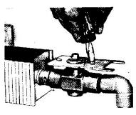
Attach the mounting plate to the valve body with the captive screws supplied. Mounting plate should be loose with screws fully seated. At this time, valve should be set in the "open" position.
