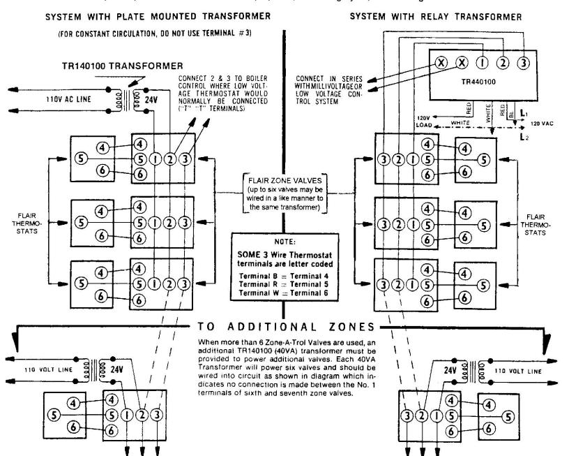
NOTE: RP044 and RP044010 replacement (5-wire) operators and thermostats with 2-wire control circuits do not have a number 6 terminal. RP024 and RP024010 use a 3-wire control circuit. Operators for VK series valves did not have a #3 terminal but are replaced with actuators that do have a #3 terminal.
