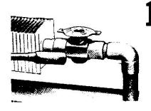
Solder valve body into supply or return side of piping. Be sure body is free of solder flux or other foreign material before stem is inserted. NPT bodies are threaded instead of soldered.
