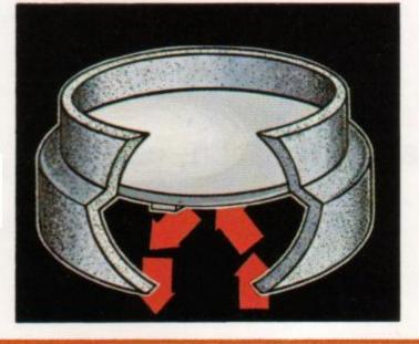
When the thermostat is satisfied, the burner goes off, and then the damper rotates to the closed position. This effectively prevents the loss of heated air through the flue from the heating appliance and from the surrounding space.
